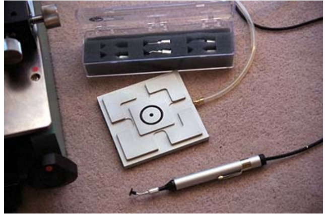
20) Vacuum wand accessory tips and spare light bulb are in accessory box.
