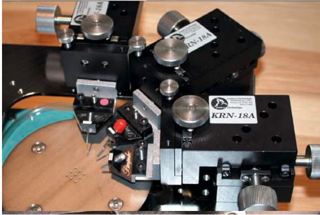
19) KRN-18 can be positioned in seven locations on top plate. (Use LDP style probes for most versatility)
