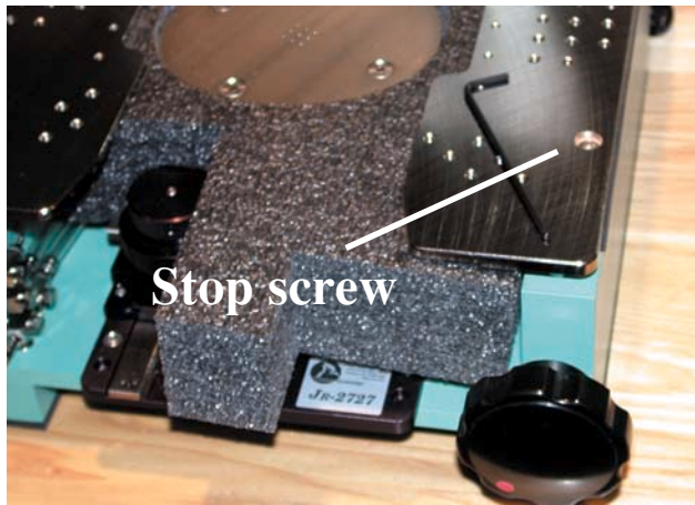
9) Loosen top plate 'stop' screw with 3/32" hex wrench. Stop screw may be removed and stored in threaded hole in rear of base.
