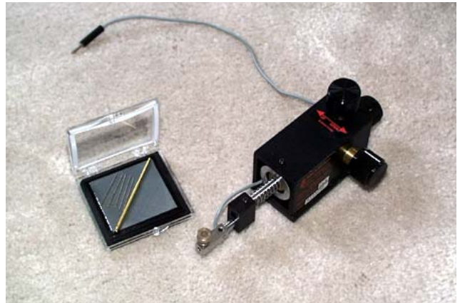
22) DC Positioner kit. Five Pd alloy needles and needle holder.
