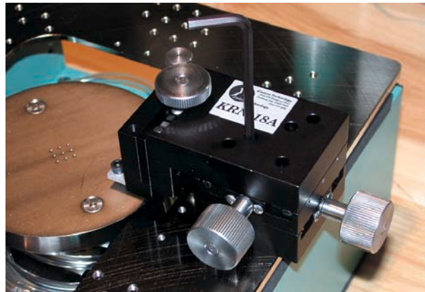
16) Mount KRN-18A using the two(2) #10 positioner mounting screws with the 5/32" allen wrench. Note: Positioner must be in 'centered' X-Y positioner to allow access to screws.
