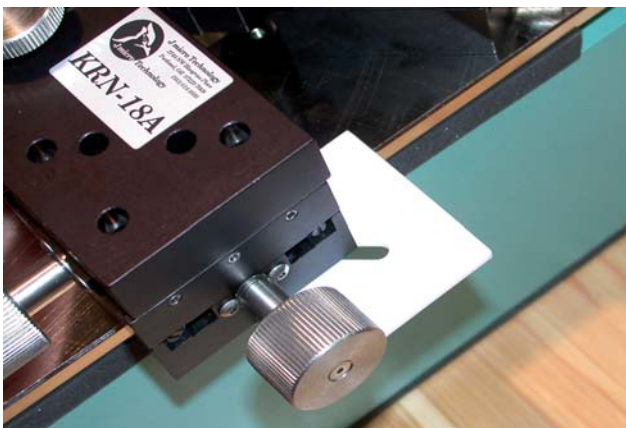
17) Positioner with PTFE spacer under body and Al spacer on probe mount. Spacer can be installed without removing positioner by loosening hold down screws and sliding slotted spacer in diagonally.
