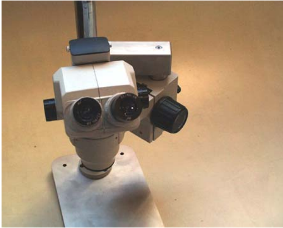
7) Mount microscope into rack on stand.
