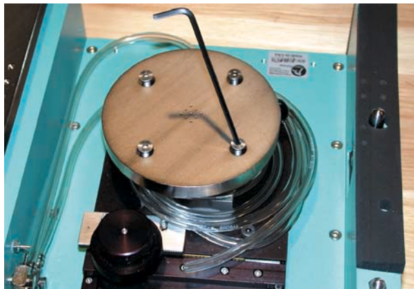
11) Remove chuck to insert spacers. Spacers are used to position the chuck plate, probe positioners or probes to accommodate various test requirements.
