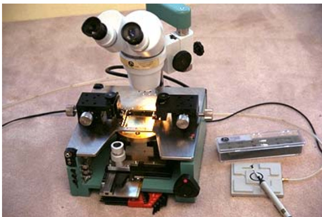
23) JR-2727 personal probe station configured for test.
