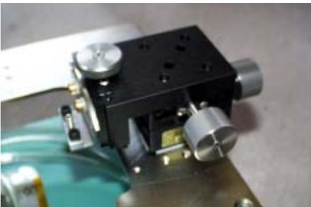
**17) Positioner may be elevated with PTFE spacer under body. Probe elevated with the Al spacer on probe mount.**
