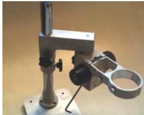
10) Position locking ring on pole, tighten. Slide swing arm assy on to pole.
