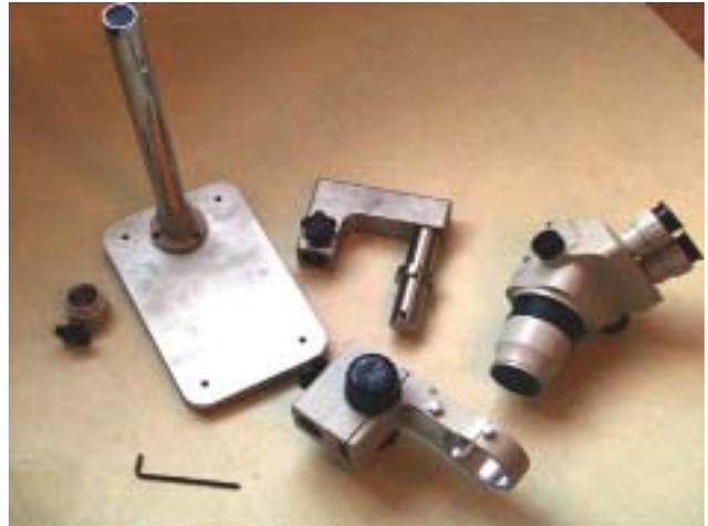
8) Remove microscope, stand, swing arm components. Remove bearing ring from end of swing arm post using 5/32 hex wrench.
