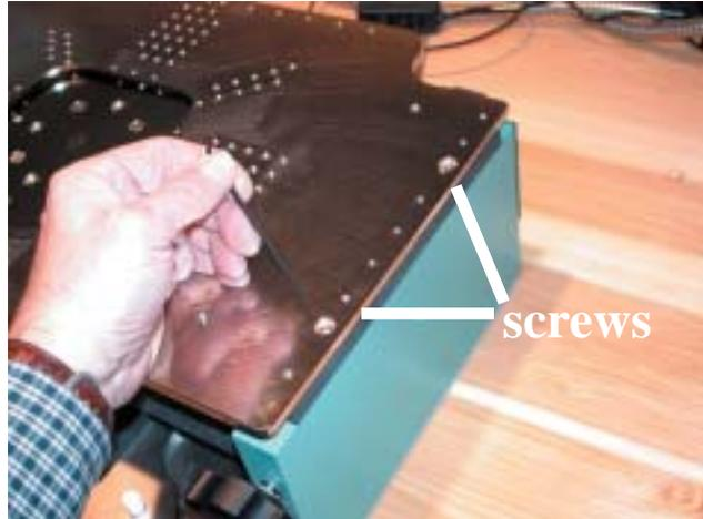
4) Loosen top plate 'stop' screws with 3/32" hex wrench.
