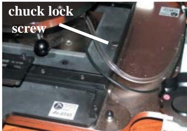
5) Raise top plate and remove chuck locking screw and store in shipping container.
