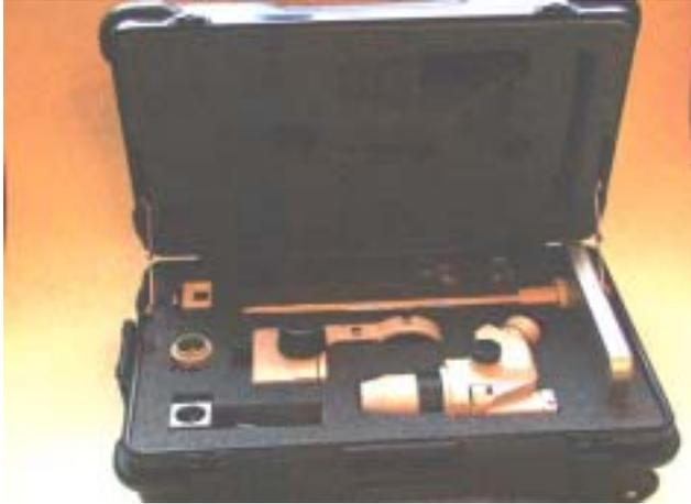
7) Probe Station is stored on in one case, optics are stored with stand in another case. Components fit snugly. Lift probe station out by grasping sides and remove slowly. Some accessories are stored under station.
