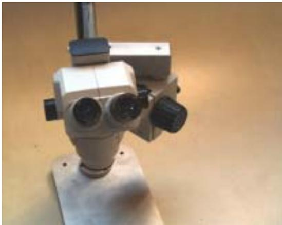
11) Mount microscope into rack on stand.
