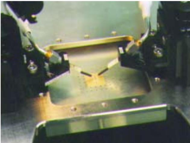
Stage in measurement position for DUT on carrier. Top plate would normally be raised prior to load/loading.
