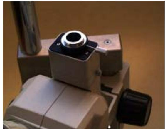
12) Option - Attach camera adapter to vertical accessor port.
