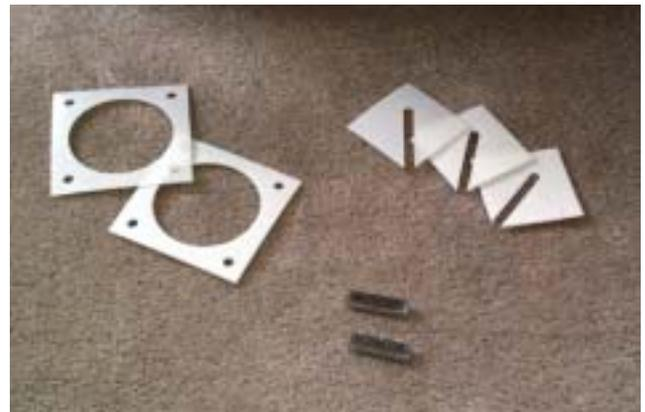
22) Spacers, from left, chuck spacers, probe spacers, positioner spacers.
