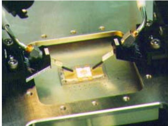
Package on carrier for measurements.
