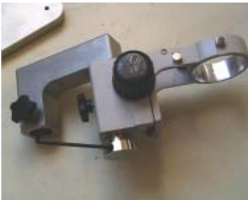
9) Slide microscope onto swing arm post. Reattach bearing ring and fasten with #10 screw(s).
