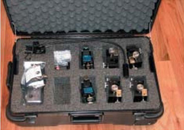
**13) Open Positioner/Accessory Box. Remove illuminator and transformer, and Positioners.**
