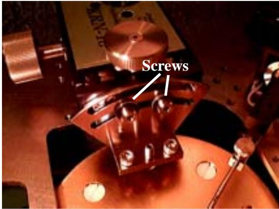
Probe planarity does not normally need to be adjusted. Loosening these screws and rotating plate will result in  $\pm 11^\circ$  of adjustability.
