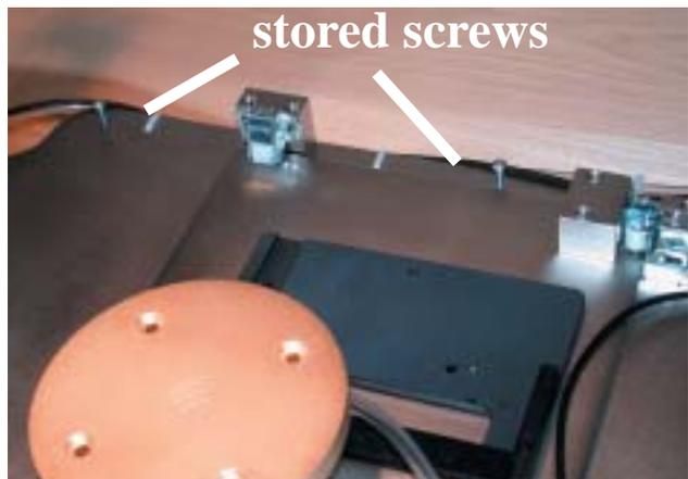
6) Stop screws may be removed and stored in threaded hole in rear of base.
