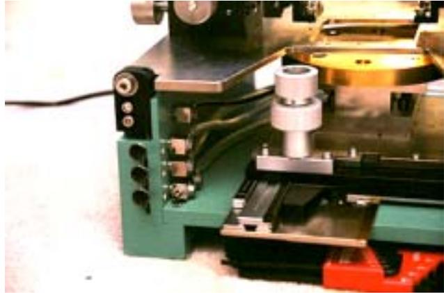
Vacuum control manifold. Upper switch is for stage. Middle switch is for vacuum release gel-pak plate. Bottom switch is unused.
