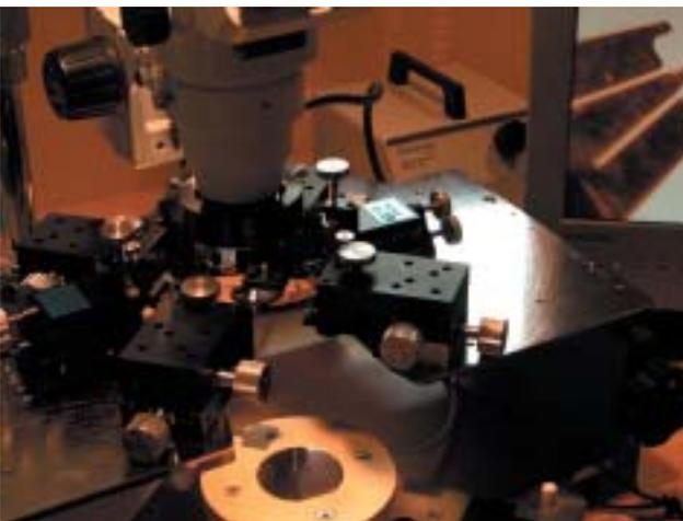
23) JR-2745 manual probe station configured for test.
