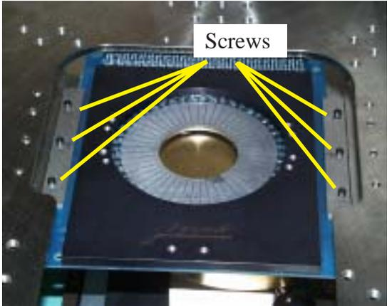
PCA1) To mount a probe card onto top plate, loosen the six(6) 2-56 socket head cap screws on the probe card clamp enough to allow probe card to slide in but still be guided by rails.
