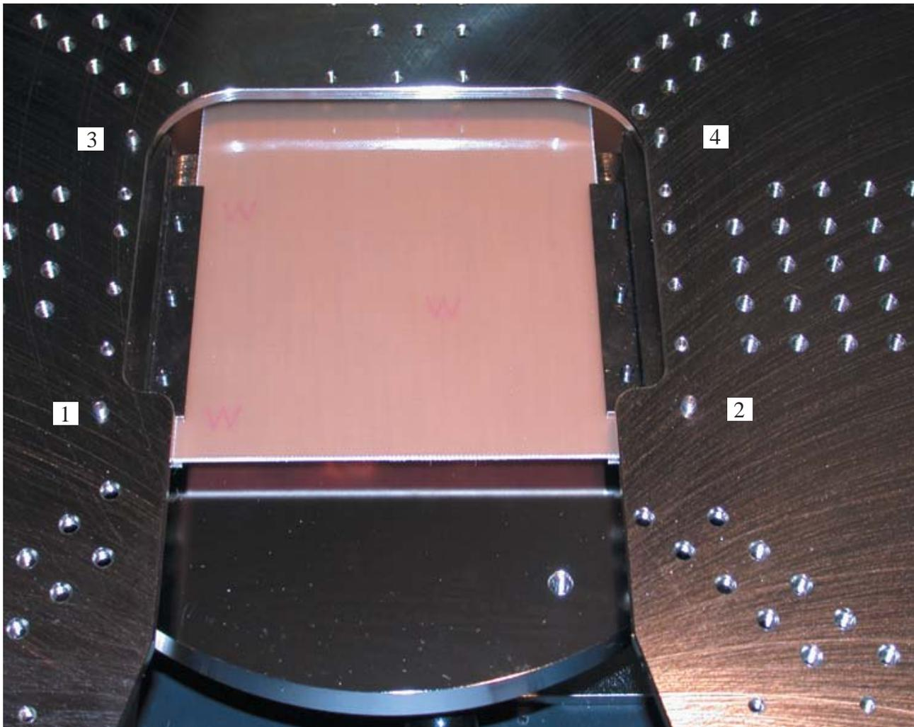
PCA7) ‘Set screws’ on left and right of probe card adjust height and planarity of probe card. Screws are approximately 30 mils per turn. Height should be set to within approximately 3 mils, or 1/8th turn resolution. The four set screws allow a 0.2” adjustability total range. That includes the depth and planarity.
