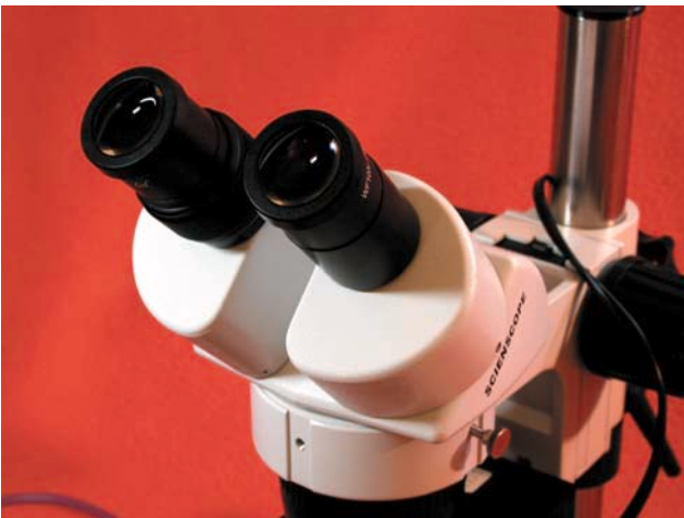
11) Install 10XWF eyepieces into microscope.
