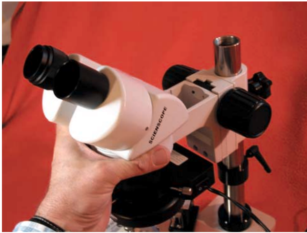
9) Mount microscope and rack onto stand.
