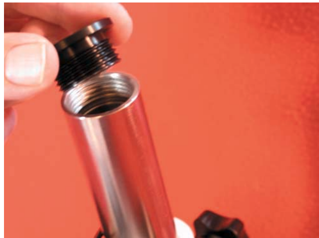
10) Install screw-in top cap on post.
