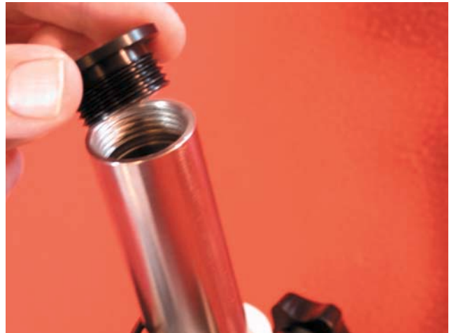
10) Install screw-in top cap on post.
