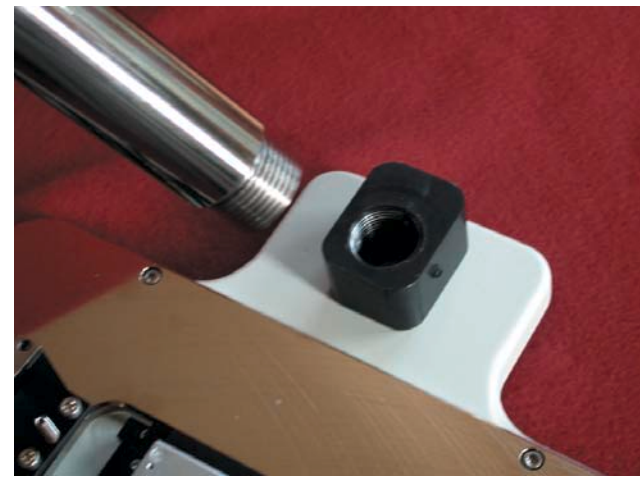
4) Install microscope stand post into black ring, hand tight. Position safety ring approximately 3" above black ring with locking handle pointed down.
