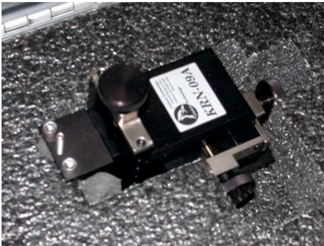
3) KRN-09A positioners are shipped and stored with x-y-z slides in 'far' position (knob screwed fully clockwise).
