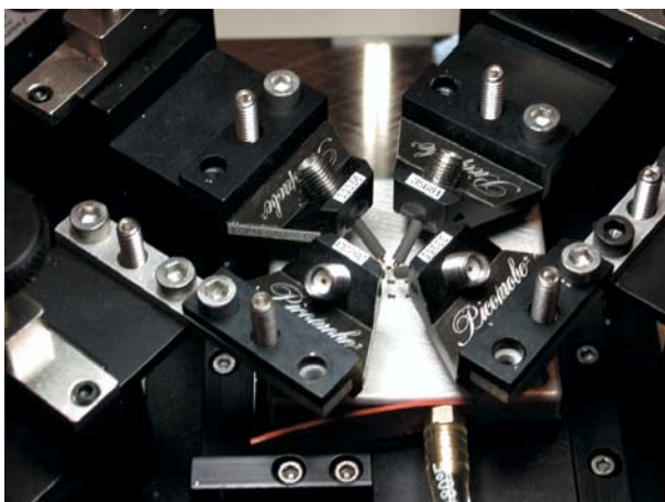
17) Four orthogonal probes are possible with 'offset' brackets
