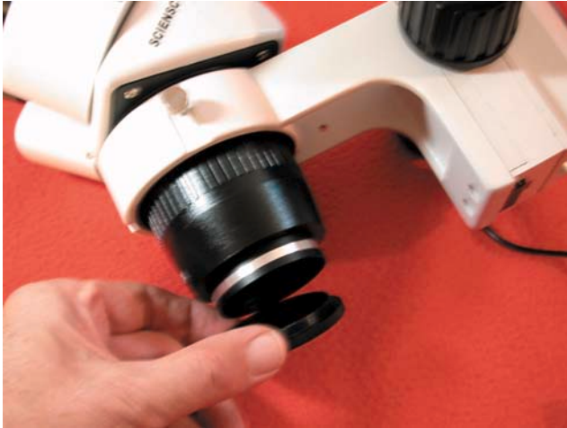
7) Remove lens cap from objective
