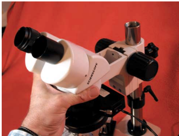
9) Mount microscope and rack onto stand.
