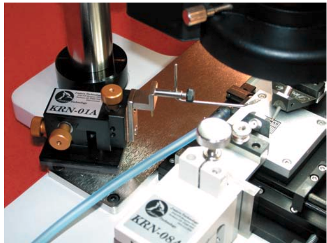
12) Optional magnetic mount DC positioners attach to platten.
