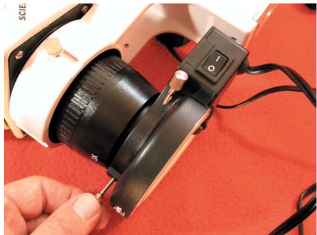
8) Position fluorescent ring illuminator on objective ring. Tighten the three(3) thumbscrews securely.
