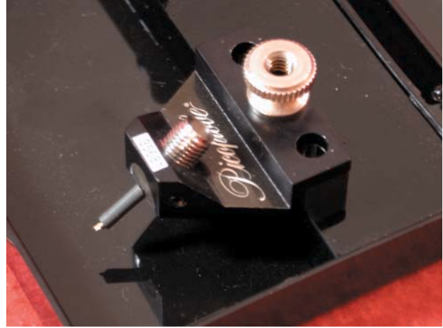
14) Open probe box and remove probe by removing 8-32 thumb nut.
