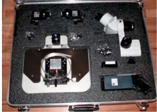
2) Begin by opening case. Remove base deck from left side of case by grasping right side of base deck by black ring and lifting out from box. Microscope stand post and fluorescent illuminator are beneath base deck
