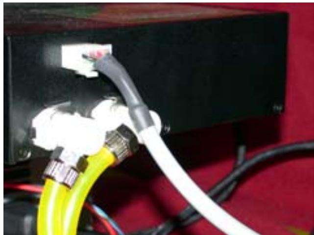
Power and water hose connection on back of Water Cooler
