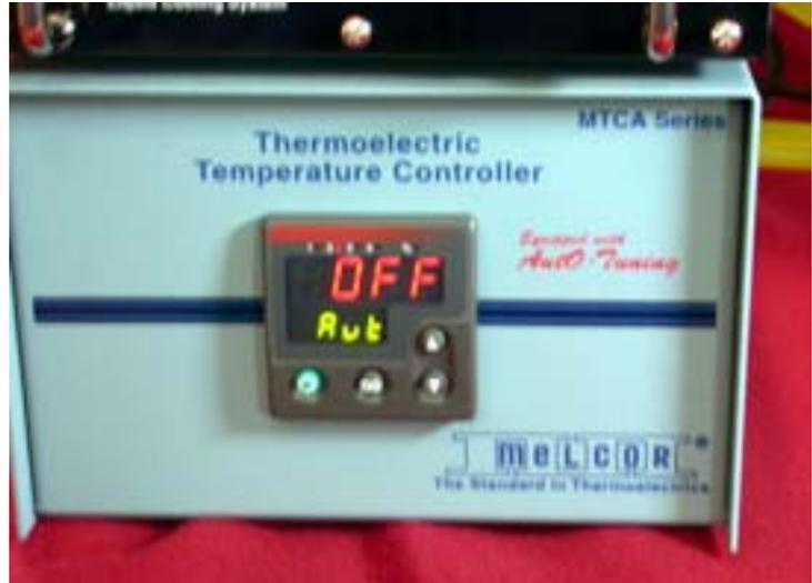
Warning. Temperature Controller default parameter settings are different from the J microTechnology default parameter settings. It is not advised that the Temperature Controller be 'reset' to factory default. A list of the specific J microTechnology setting modifications is listed in appendix A, if that is ever required
