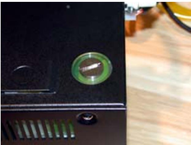
Reservoir fill/drain plub on bottom of Water Cooler
