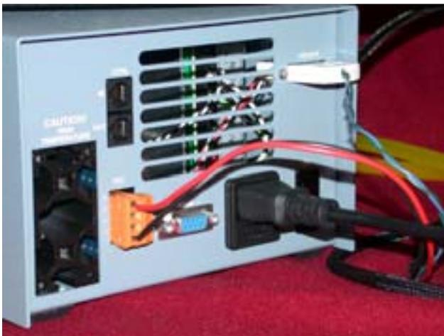
Temperature Controller is operational at this point. Do not turn on and operate for more than 1-2 minutes without the Water Cooler connected.
